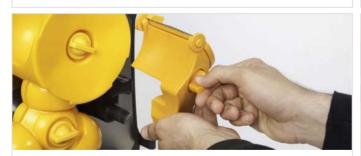
**11.** Insert the twirler blade and support and place the security lock in disassembly position.
