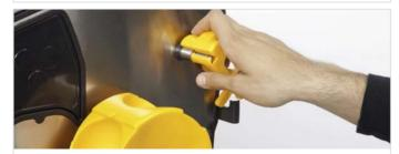
**13.** Place the retainer in the axis, make sure it is correctly fitted can move smoothly.
