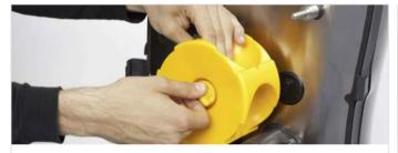
9. Tighten the securing knobs of the squeezing units.
