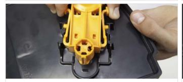
17. Release the tap by pressing its sides to loose the pins.
