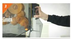
Take out the cover sides. **Press** the button / extract the peel guides.
