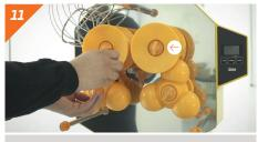
Unscrew the securing knobs of the pressing units.
