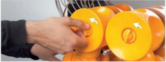
**6.** Unscrew the securing knobs of the pressing unit.
