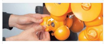
**13.** Fix the knobs and tighten them well. Missing knobs are to be replaced immediately. Never operate the machine with any knob missing.
