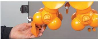
**14.** Put on the peel ejectors. Push them firmly to assure their right positioning in order to avoid breakage while using the machine.
